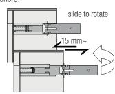
Snap the cover onto the hinges. Close it and secure it using the supplied screws. After the settings and adjustments, fasten the cover using the supplied screws.
