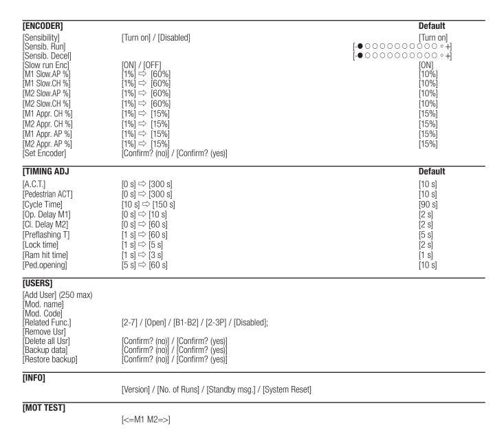
IMPORTANT! Start programming by first executing the following functions [MOTOR TYPE][NO. MOTORS], [TOTAL STOP] and [SET ENCODER] function.
