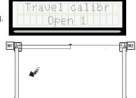
7. Once the procedure is completed, the display will read [Travel calibr OK] for a few seconds.
