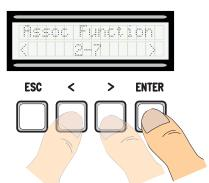
4. ... a code to enter will be requested. Send the code from the transmitter, with the swipe card or transponder.
